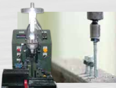
AS3566 Drilling Test
