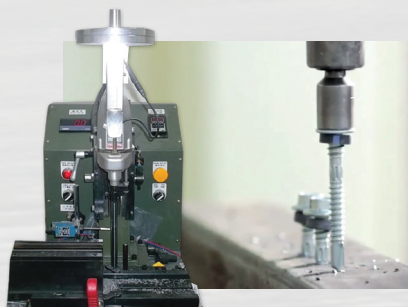
AS3566 Drilling Test
